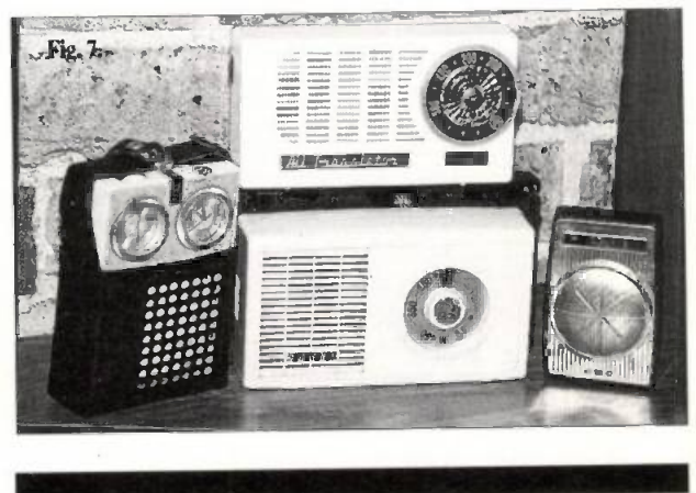
Fig. 7: Collectable transistor receivers. (Left) the Russian-made 'Signal 601 with wind-up watch type alarm. The Ekco (bottom) tunes through the medium wave band and 'clicks' into a preset 'Light' programme on the long waves (now BBC Radio 4).
