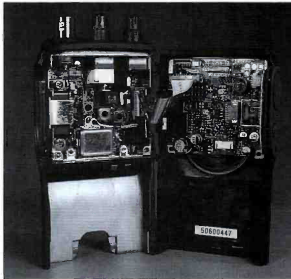
Fig. 1: Internal view of the Kenwood TH-22E 144MHz transceiver, clearly showing that the battery pack takes half the available space on this extremely light and very portable hand-held.
