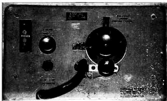
Fig. 2: The receiver chassis of the 18 set showing interconnecting h.t./l.t. connecting lead (see text).
