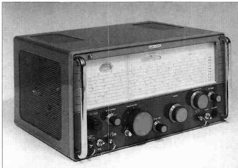
Fig. 2: The later Model 830 300kHz to 30MHz receiver employed a steel case.
