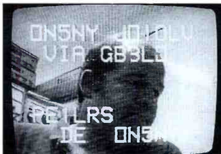
Fig. 1: Talk about the long way round! Here's PE1LRS working ON5NY by way of GB3LO, the amateur television repeater in Lowestoft.
