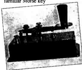
Fig. 1: The Marconi key. The base contains a capacitor for spark reduction (see text).
