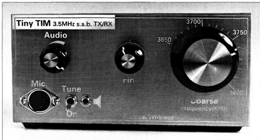
The PW production prototype Tiny TIM as built by Tex Swann G1TEX and tested on air by G3XFD. The front panel uses p.c.b. material (see text).
