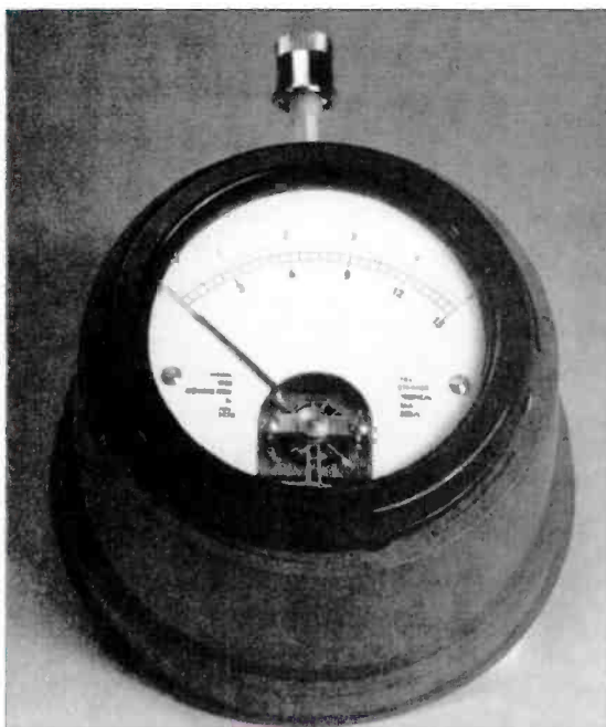
Fig. 3: Using G3KKC's method of extending the current ranges of low current reading meters, such as the one in the photograph, (which cost £1 at a rally) can prove to be excellent value-for-money.
