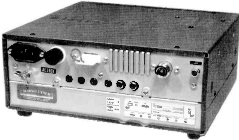
The rear panel of the IC-R7100HF clearly demonstrates the many facilities provided on this receiver.
