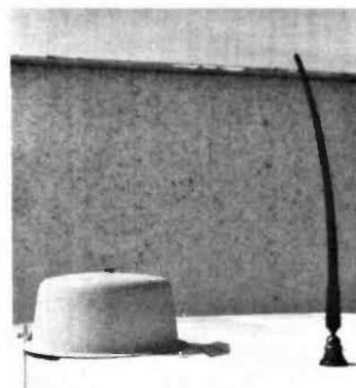
The 'Untenna' mounted on a Luton-bodied van next to a standard flexi-type car radio antenna.
