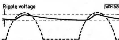
Fig. 5.5: Ripple voltage across the reservoir capacitor for a half wave rectifier
