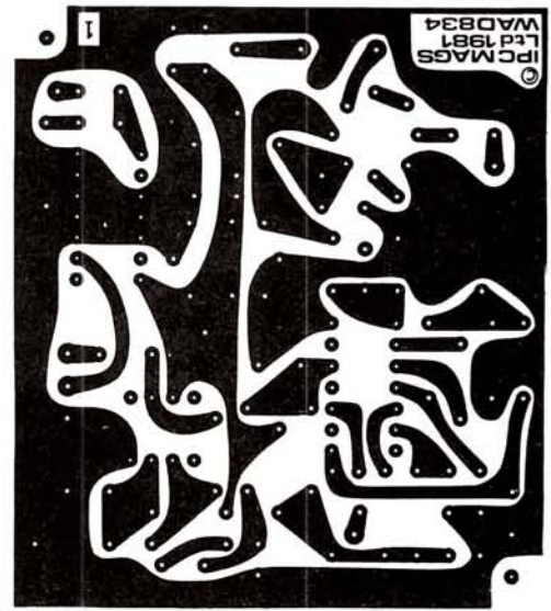
Fig. 3 (above): Full size track pattern of the underside of board 1
