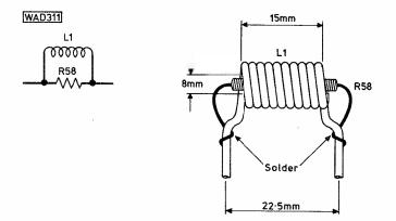
Fig. 6: Winding details of the two coils L1. Internal diameter 8mm; Length 15mm; 3 layers of 10 turns each (Total 30 turns) 18 s.w.g. enamel copper wire. R58 is  $10\Omega$  1W carbon resistor
