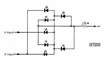
Fig. 4: Circuit diagram of one l.e.d. display. This forms the display for one square and nine of these are required for the complete game. The  $270\Omega$  resistor is the approximate value needed to limit total current to 10mA
