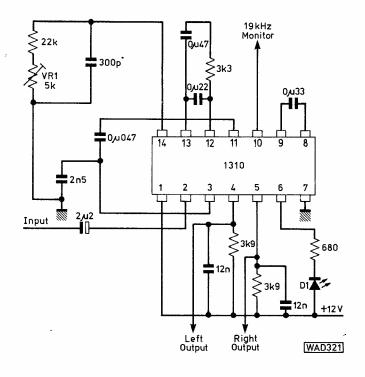
Fig. 3: External circuitry required for the MC1310
