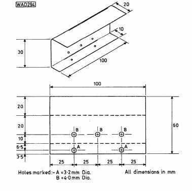
Fig. 5: Construction of the tinplate screen
