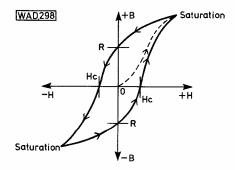
Fig. 1: Hysteresis loop of magnetisation. See text for description
