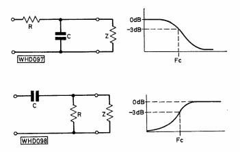
Fig. 1: Basic filter circuits and their response curves: (a) (Top) Low-pass. (b) (Bottom) High-pass
