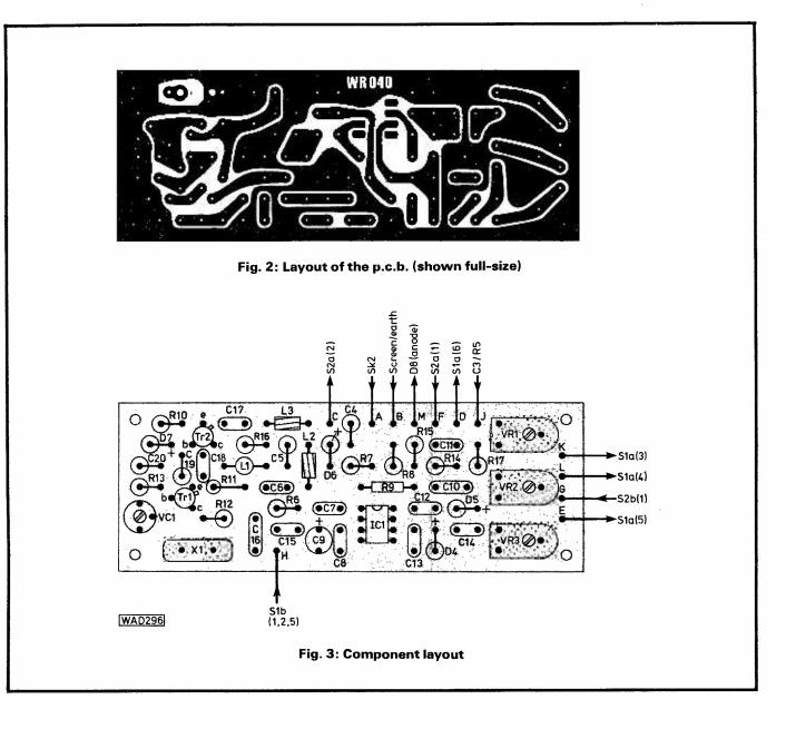
this frequency is used (8.08333MHz for 145.5MHz, for instance), Tr2 multiplies 18 times, L1, together with the stray and internal capacitance of Tr2, resonating at approximately 145.000MHz.
