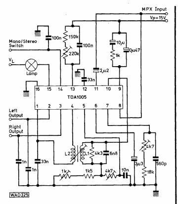
Fig. 7: External circuitry for the TDA1005 in the frequency multiplex mode
