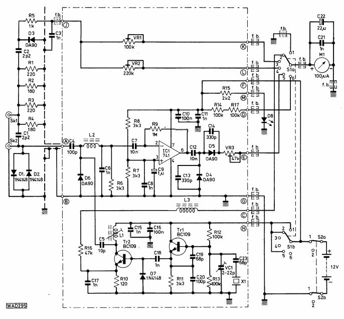
Fig. 1: Circuit of the Multitester
