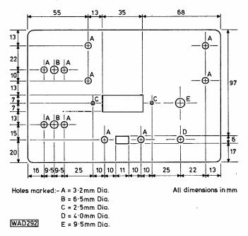
Fig. 4: Drilling details for the box lid
