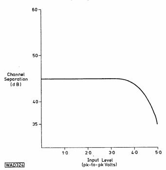
Fig. 6: Channel separation plotted against input signal level
