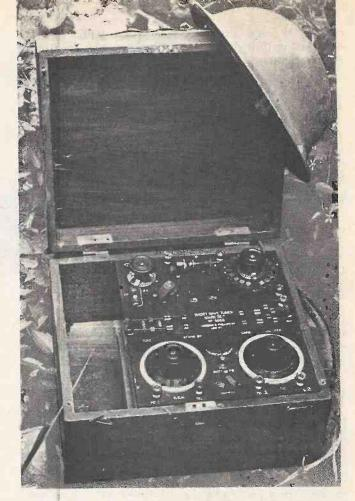
Fig. 3 Short-wave Tuner, Mark III made by Johnson and Philips
