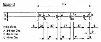
Fig. 12: Above, details of the control mounting bracket which is made from 1.2mm thick aluminium
