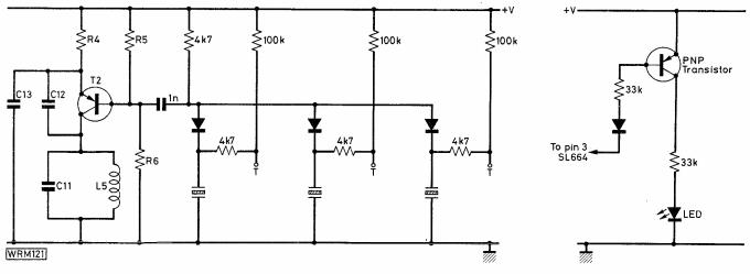
Fig. 2 (left): Adding multi-channel facilities. Grounding one terminal ''T'' activates the associated crystal Fig. 3 (right): Driving a l.e.d. squelch indicator requires this simple buffer stage
