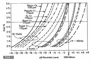
Fig. 3: Curves showing how the distortion increases at three different frequencies as the recorded level and hence the tape flux is increased. The results represent the averages of a number of samples and batches of the tape types indicated, when used with domestic cassette decks
