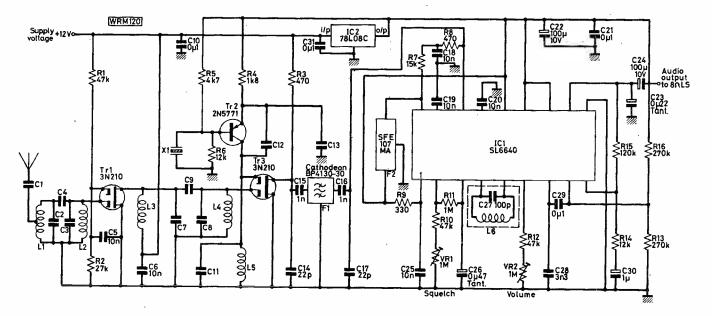
Fig. 1: Complete circuit diagram of the single-channel version of the receiver
