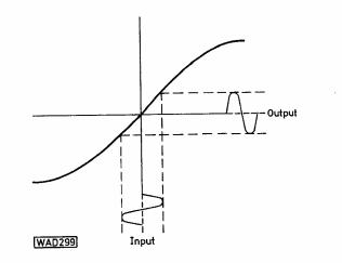
Fig. 2: Transfer characteristic of magnetic tape showing non-linearity of odd-order terms, which is responsible for odd-order distortion on the output signal. The curve takes account of the correction provided by the h.f. bias
