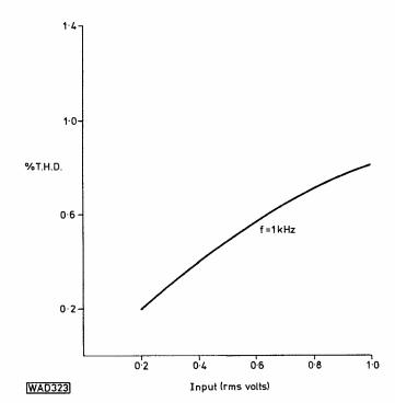
Fig. 5: Relationship between total harmonic distortion and input signal level
