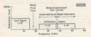
Fig. 1: Spectrum of the stereo multiplexed signal
