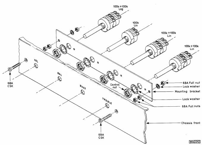
Fig. 15: Method of mounting the control potentiometers using the pot mounting bracket
