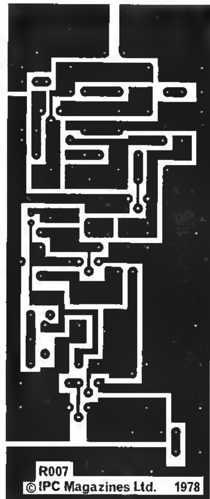
Fig. 6: Copper track layout for Board 1. Ready drilled boards for this instrument are available from Reader's PCB Services (See page 68)
