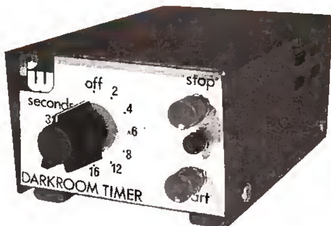
The timer is built into a small instrument case with all the controls on the front panel
