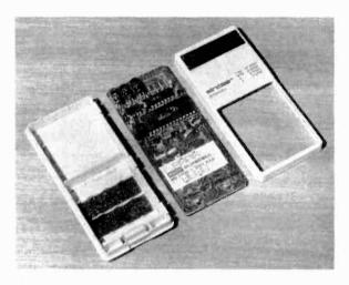
The two case halves snap together to secure the p.c.b. A door in the back section covers the battery compartment.
