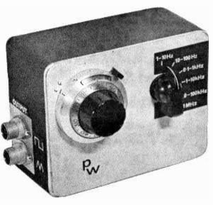
▲ The finished waveform generator with its direct reading dial. The necessary components to produce a ramp waveform can be added to the circuit board. For converting triangular waveforms to sinewaves a separate unit is required.
