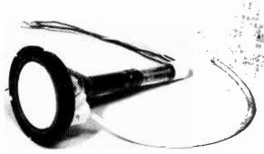
The 700J projection CRT is designed for use with high brightness head-up radar displays and requires an anode voltage of 15kV. This tube is also a M-O Valve Co. product.
