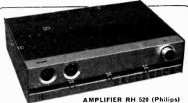
Successor to the 590, this  $2\times15W$  r.m.s. amplifier conforms to DIN 45500 Standard. It has switchable "Stereo-4" quadraphonic facility, rumble and scratch filters, slider controls, headphone socket, power meters. Recommended retail price £85 including VAT
