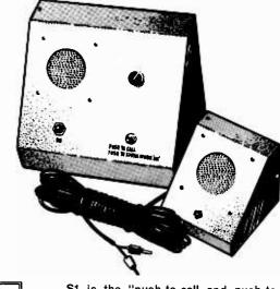
S1 is the "push-to-call and push-to-speak" switch. When it is pressed, the circuit is completed in such a way as to cause an audio tone (R1 limits current in this condition). S2 switches the unit on so that the master position may speak to the remote position, or vice versa. S3 at the remote unit causes a tone at the master unit, to gain attention.
