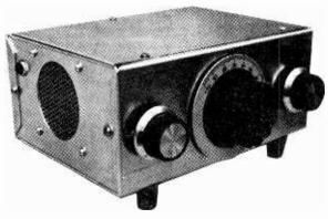
This view of the receiver shows the positioning of the internal loudspeaker and the socket for an external loudspeaker or headphones.
