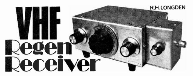
THIS is a self-contained receiver which may be used over the range 115-150MHz, or 140-190MHz, according to the coil fitted. It was actually found to maintain good efficiency even up to 210MHz. A vertical telescopic aerial or improved aerial system will provide reception on the internal speaker, an outlet being present for headphones when required. An optional preamplifier is also described.
