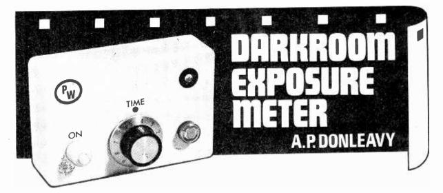
THIS instrument was designed for use with a photographic enlarger, to determine the exposure required for any particular print. It is cheap to build and easy to use, with a range up to about 40 seconds.
