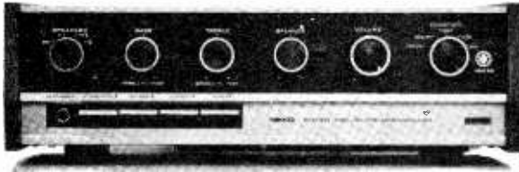
The Nikko TRM-50 amplifier built up around ICs.
