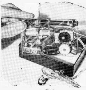
D1 through C1. The detected audio is then returned to the base of T1, to be amplified once more, through C3. The audio output is developed across R4, and C6 feeds the audio signal to T2 for final amplification. The output is loud enough for most purposes, although further
