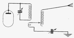
Fig. 4.—The series tuned Marconi aerial corresponds to the artificial aerial equivalent shown in Fig. 2.
