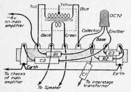
Fig. 45.—Wiring diagram of the audio stage.
