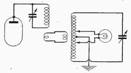
Fig. 6.—The artificial aerial parallel tuned circuit arranged to simulate a parallel tuned twin wire feeder system.
