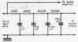
Fig. 3.—The low-pass filter which is employed.
