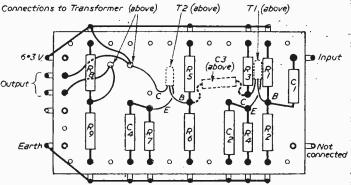
Fig. 47.—Tagboard layout of the audio amplifier,
