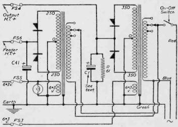
Fig. 3.—Circuit of the power supply.
