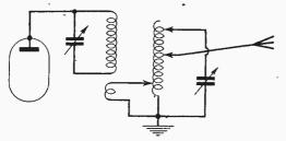
Fig. 5.—The end fed parallel tuned aerial system is the real life equivalent of the artificial aerial of Fig. 3.
