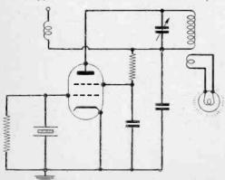
Fig. 1.—An inductively coupled lamp load is one of the simplest output indicators.
