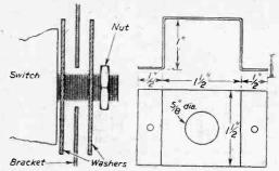
Fig. 4.—Details of wavechange switch mounting.
