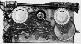
A plan view of the finished receiver.
