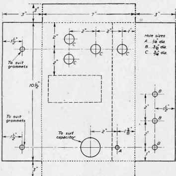
Fig. 4.—Output chassis main dimensions.
