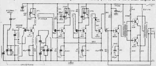
Fig. 1.—Circuit of the Ace transistor portable.
