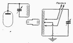
Fig. 7.—Radiating aerials with twin wire feeders are fed in this manner from a parallel tuned circuit.
