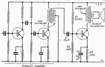
Fig. 44.—Circuit of the complete amplifier.
