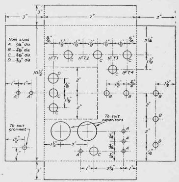
Fig. 5.—Drilling details for the feeder unit chassis.
