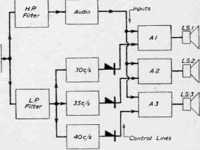
Fig. 1.—Block schematic of a professional form of single track recorder.
