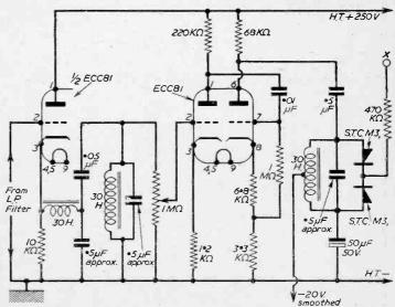
Fig. 4.—The professional circuit of the sub-carrier filter unit.
