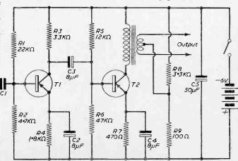
Fig. 46.—A two-stage audio amplifier with output base potentiometer.
