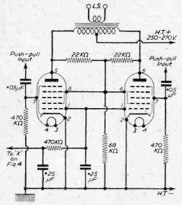
Fig. 2.—Circuit of the output stage of the recorder.
