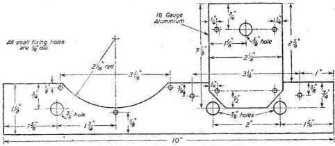
Fig. 3.—Details of the front of the chassis.
