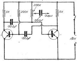
Fig. 2.—The transistor form of Fig. 1.
