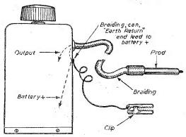
Fig. 4.—The completed oscillator in its case.
