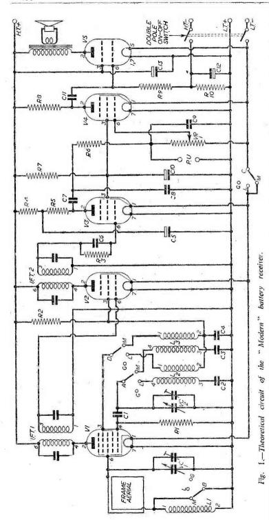
strength can be so obtained because the volune control will then be nearer maximum for a given volume of signal; in other words the detector will be working on a smaller signal which will be better for quality.
