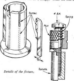
similarly, cutting one slot midway between two keys. Assemble the nut on the spindle with a light spring seating in the larger hole in the top of the nut, a 4 B.A. screw in the spindle retaining both.
