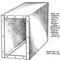
Fig. 6.—Details of the case.
