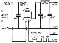
Fig. 3.—The A.C./D.C. version of the power-pack.
