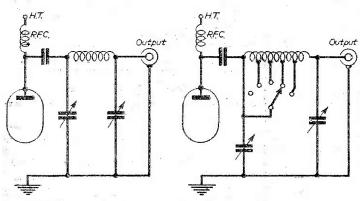
Fig. 1.—The basic PI tank circuit arrangement.
