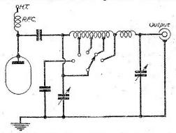
Fig. 4.—The L/C ratio required for 80-metre operation can be achieved by switching in an auxiliary fixed capacitor across the main tuning capacitor. This enables the main condenser to be a convenient size for comfortable tuning of the higher frequency bands.
