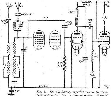
broken down to a two-valve mains version. Some of the parts are retained, and the new parts are shown in heavy lines.
