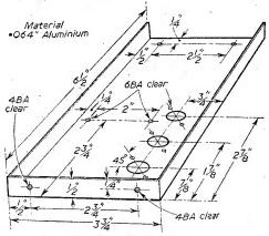
Fig. 3.—Details of the chassis.
