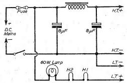
Fig. 2.—The complete power-pack, showing how the mains may be adapted to the leads of the battery set.
