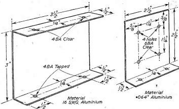
Fig. 2.—Details of rear bracket (left) and coil bracket (right).
