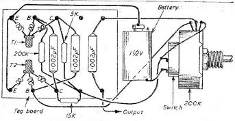
Fig. 3. - Wiring diagram of the oscillator.
