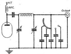
Fig. 7.—Fine and coarse loading control by means of a small variable capacitor in combination with a switched bank of fixed mica capacitors.
