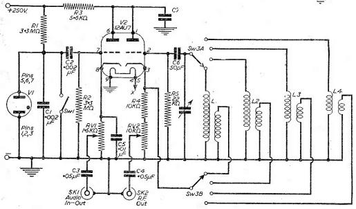
Fig. 1.—Theoretical circuit of the generator, with the mains section above.
