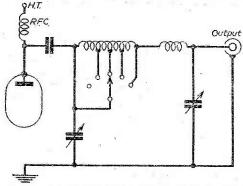
Fig. 5.—A TVI trap circuit resonated to the local TV channel may assist in reducing harmonic radiation when the PI tank itself does not give adequate harmonic supression.
