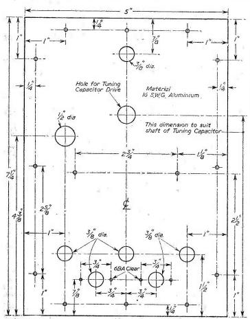
Fig. 7.—Front panel details.
