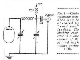
also heat up appreciably. Adjustment of the choke turns and spacing may enable the trouble to be cured, but remember that wrong adjustment may throw the deleterious resonance into an adjacent H.F. band. There are chokes commercially available designed for PI tank service, but in some cases the amateur may already own a large transmitting choke of the older type which gives trouble in PI tank service.
