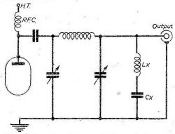
Fig. 6.—The series resonant combination Lx and Cx is tuned to the local TV channel to remove harmonic radiation from the PI tank output. An anode circuit trap may also be used in conjunction with the above "gimmick."
