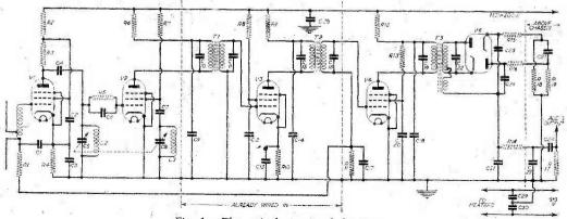
Fig. 1.—Theoretical circuit of the tuner,
