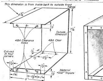
Fig. 5.—The containing case body.
