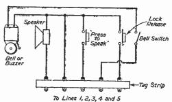
Fig. 4 (a)—Flat unit wiring.
