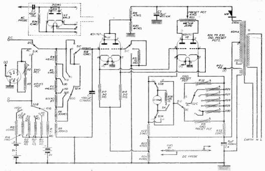
Fig. 1.—Theoretical circuit of the Meter. R and C details are given and the remaining components cre listed on page 664.
