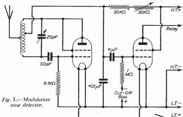
bias and wiring phones from anode to H.T. positive. The receiver is then carried to a distance (preferably at least 50 yards from the transmitter) and adjusted for maximum volume in the phones. These adjustments will consist of tuning, modification of aerial and H.T. feed coil tappings, and adjust-ment of the 50 K oscillation When maximum volume is obtained just sufficient bias is applied to prevent the second valve conducting, with transmitter off.
