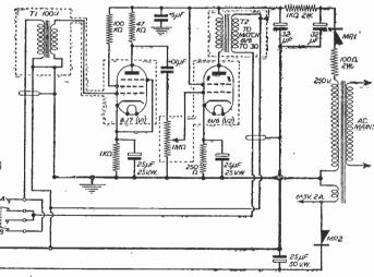
Fig. 1.—Complete circuit of the novel inter-com. Illustrations of the door and room units will be found on page 683, whilst the list of parts for the amplifier appears on page 686.
