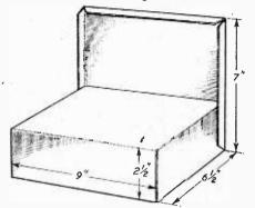
Fig. 4.-How the chassis is made up.
