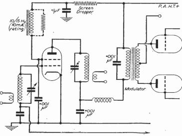
Fig. 4.—The self screen modulator rigcuit reproduced from last month's issue,
