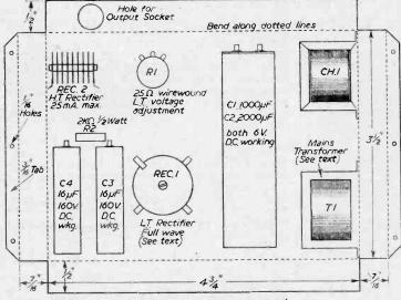
Fig. 2.—Layout and component values.
