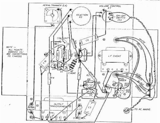
Fig. 6.—Below chassis wiring details.
