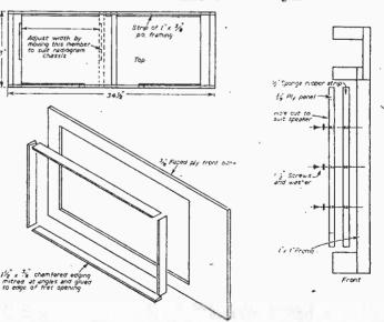
Fig. 6. -Boffle, front and further constructional details.
