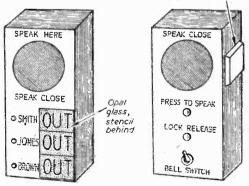
Fig. 2.—Details of the front door (left) and the room units (right).
