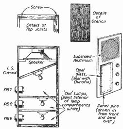
Fig. 3.—Constructional details of the front door unit.
