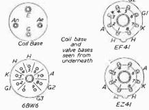
Fig. 7. - Details of valve base connections.
