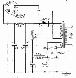
Fig. 1.—Theoretical circuit of the unit.
