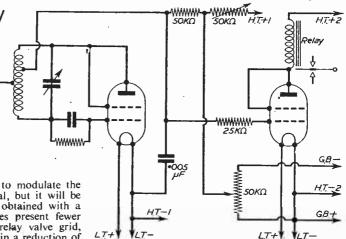
Fig. 4.—Direct-coupled amplifier.
