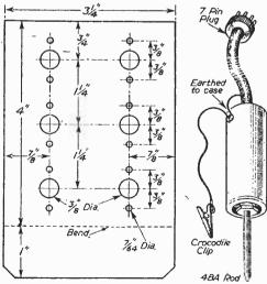
Fig. 7.—Drilling and bending details of the potentiometer bracket.
