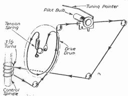
Fig. 4.—Details of the dial drive.
