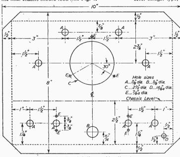
Fig. 2.—Panel drilling and bending data.
