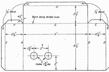
Fig. 3.—Chassis bending and drilling data.
