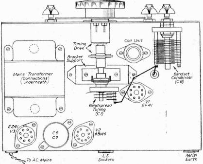
Fig. 5.—Above chassis wiring and layout details.
