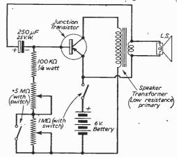
Fig. 1.—Theoretical circuit of the Metronome.
