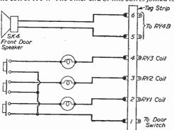
Fig. 4 (b)—Door unit wiring.
