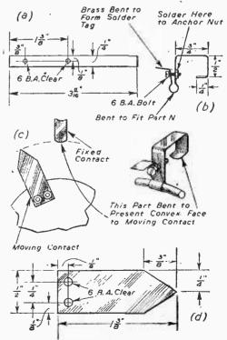
Fig. 21.—(a) and (b). Details of fixed contacts. (c)
