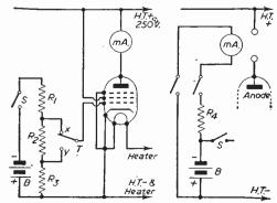
Figs. I and 2.—The circuit diagram and method of arranging battery check.
