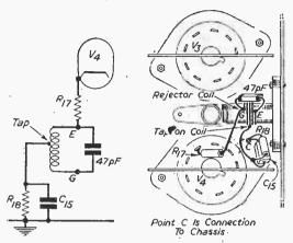
Fig. 2.—Position of the rejector coil in the cathode circuit of V4.
