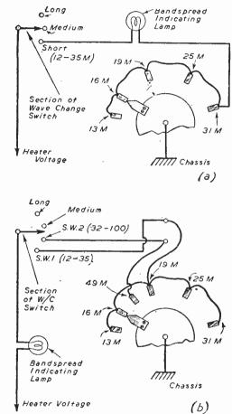
Fig. 23.—(a) and (b). Various methods of connecting the fixed contacts and bandspread indicating lamps to obtain different effects.
