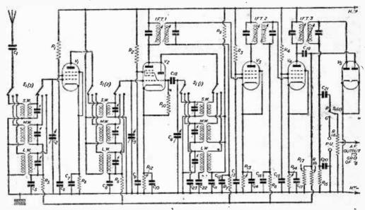
Fig. 1.—Theoretical circuit of the receiver.
