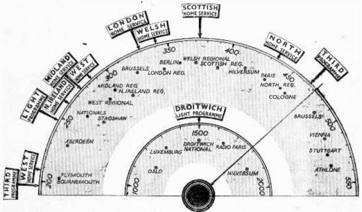
Appearance of the standard Tuning Dial showing positions of the B.B.C. stations under the new plan.
