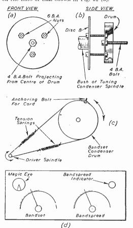
Fig. 22.—(a) and (b). How a drum for a cord drive may be fitted to the bandset tuning condenser. (c) A spring is fitted to both sides of the cord drive to avoid strain (see text). (d) Suggested dial layout for the unit.
