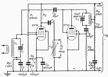
Fig. 1.—Typical television mixer circuit.
