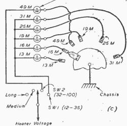
Fig. 23.—(c). Further method of connecting the contacts.
