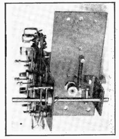
Fig. 24.—View underneath the unit. The D.P.S.T. switch mechanism is clearly visible. ("Condenser free" position, switch open.)
