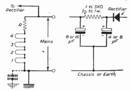
Fig. 1 (left).—Normal arrangement of heaters for A.C. or D.C. supply. Fig. 2 (rig!it).—H.T. smoothing at its simplest,
