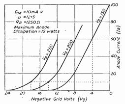
Fig. 1.—Characteristics of a heavy-duty triode valve.
