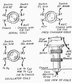
Fig. 4.—Coil connection details.
