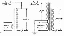
Fig. 3 (left).—Using a transformer for the heater supply. Fig. 4 (right).—Isolating the receiver from the mains by a single transformer.
