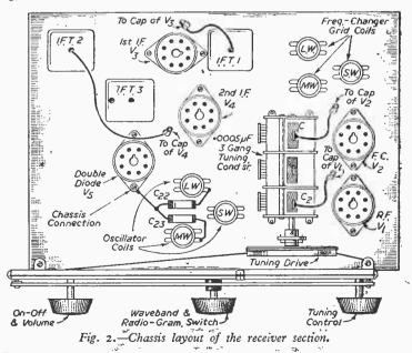
Some makes of I.F. transformers may have a different method of colour-coding, and this should be watched. As a rule it is quite easy to see which pairs of leads are common to the transformer windings; if not, a test for continuity will reveal this.
