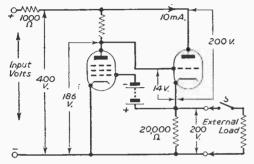
Fig. 3.—A high-gain pentode added to the circuit of Fig. 2.
