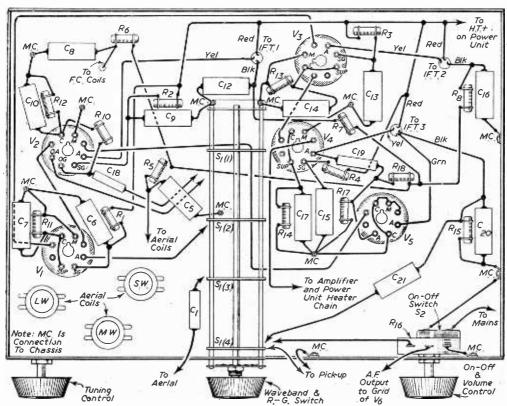
Fig. 3.-Wiring details of the receiver section. The amplifier portion will be dealt with next month.
