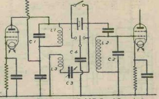
Fig. 2.- A simple single neutralised I.F. Crystal Stage circuit.
