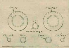
Fig. 5.-Layout of the panel controls.
