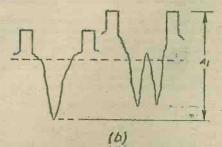
Fig. 17.—Vision signals with the D.C. component retained at (a) do not constitute such an uneconomical grid swing as those with the D.C. component removed as at (b).
