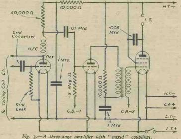
preference when this is done. If the transformer is of the type suitable for including directly in the anode circuit then the primary should be connected in place of the 40,000 ohm resistor shown. The 10,000 ohm decoupling resistor may then be taken to a H.T. tapping of about 80 volts.
