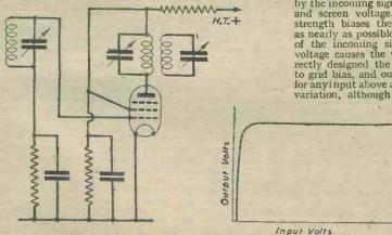
Fig. 1.—Skeleton circuit of a saturated-amplifier amplitude limiter, and on the right a diagrammatic performance curve.
