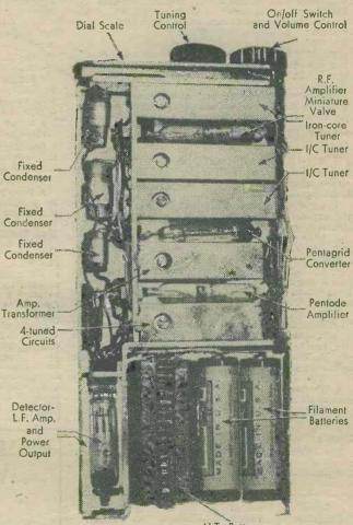
Interior of the new Belmont Pocket Radio Receiver. This measures 3in. wide, 64in. high, and is only in. thick. It weighs 10 ounces with batteries. The complete set may be seen on page 443.
