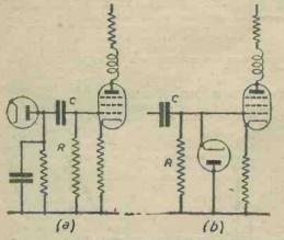
Fig. 16.—A resistance-coupled video stage at (a) with a D.C. restoration diode connected at (b).
