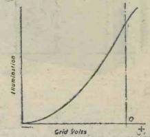
Fig. 19.—Due to non-linearity of the tube grid-brilliance characteristic the picture loses contrast in the dark regions.
