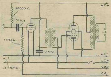
Fig. 5 .- This two-stage amplifier uses a Class B valve.
