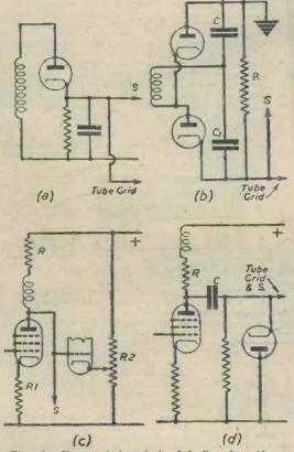
Fig. 18 .- Four typical methods of feeding the grid of the cathode-ray tube with the vision signals.
