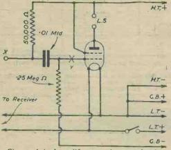
Fig. 1.—A simple amplifier stage using a tetrode valve.
