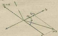
Fig. 7 .- Vector diagram for load having resistance and capacitive reactance.
