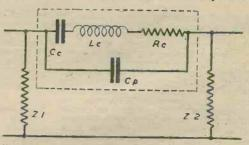
Fig. 4.-Theoretical representation of the circuit of Fig. 2.
