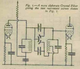
A similar result may be obtained by lowering the impedance of one or both of the side circuits by inserting series damping, but the crystal filter stage then has substantially lower gain.
