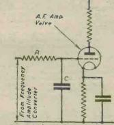
Fig. 2.—De-emphasis can be accomplished by a single top-cut filter, R and C.
