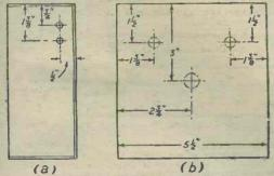
Fig. 2.—Cabinet side and front, with drilling details.
