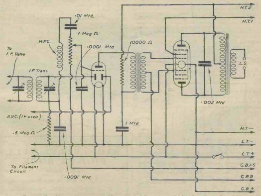
Fig. 6.—An elaborate two-stage amplifier, with Q.P.P., and a multiple value for the first stage.
