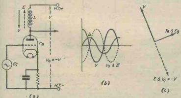
Fig. 2.—With a pure inductance L in the anode circuit, there is a back E.M.F., E, which requires a "supply" component V equal and opposite to it. The anode-to-cathode valve voltage, Vo, has the same phase as E, i.e., both have a negative sign, relative to V.
