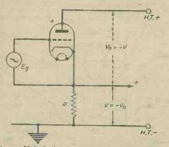
Fig. 3.—If the load resistance R were put on the cathode side, the output voltage would be V = -Vo. There is no phase-reversal such as exists across the value.
