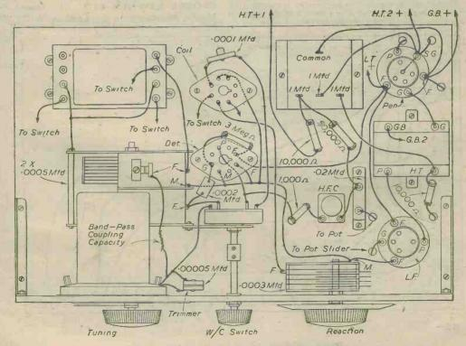
Fig. 2.- Above chassis wiring of the All-wave Three:
