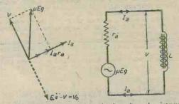
Fig. 5.—Equivalent valve circuit, when the internal resistance ra is taken into account (purely inductive load).
