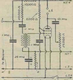
Fig. 2.—A parallel-fed transformer-coupled amplifier.
