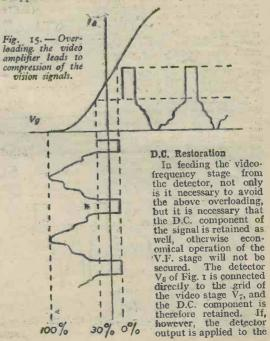
video-amplifier through any form of resistance-capacity coupling, such as is shown in Fig. 16a, the condenser C will remove the D.C. component of the signal and proper working of the video stage will not be obtained.
