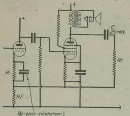
Fig. 3.—An improved version of Fig. 2. Both sides of the potentiometer can now be varied.
