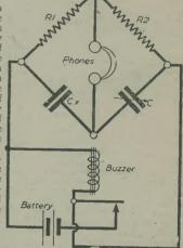
Fig. 2.—The essentials of a capacity bridge for measuring the capacity of the condenser marked Cx. Condenser C is a variable one with an accurately calibrated scale.
