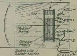
Fig. 2 .- A plan of the instrument. Note the location of the compass needle, the pointer and scale.
