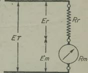
Simple method of calculating the resistance of a voltmeter, as described in H. Wiener's letter.
