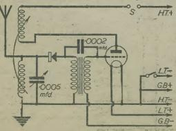
Fig. 2.—A suggested circuit using valve and crystal; the former acting as, L:F. amplifier
