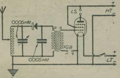
manufac- Fig. 1.— A normal crystal detector circuit followed by a pentode that a L.F. stage. A good set for reception of the local transmission, for inputs but a high degree of selectivity must not be expected.
