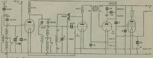
Fig. 14 .- The theo. of the £5 5s. Battery Four, blueprint No. W.M. 381. This is a good general purpose dual-range receiver.
