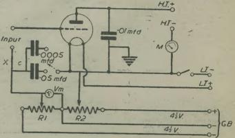
Fig. 1.-The simplicity of the value voltmeter is shown by this theoretical diagram.
