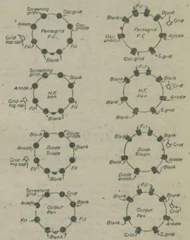
Value-base (underneath) connections for 1.4-volt octal (left) and side-contact (right) values.
