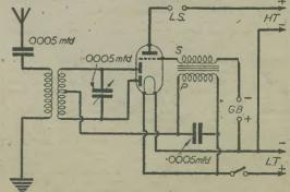
Fig. 3.—Using a D.D.T. valve as diode detector and triode L.F. amplifier.
