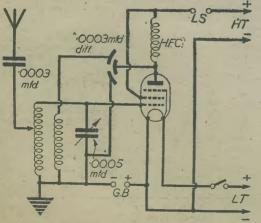
Fig. 2.-An anode-bend detector arrangement, which utilises a steep-slope pentode.
