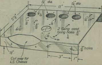
Fig. 2. - Chassis diagram showing positions of holes for valueholders, etc.
