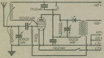
Fig. 1.—The circuit of a pentode-crystal combination in which the value acts as an H.F. and L.F. amplifier.
