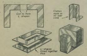
An easily constructed microphone transformer.
