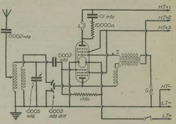
Fig. 4.—The two pentode sections of a Q.P.P. valve are used in this circuit as detector and L.F. stage.
