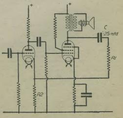
Fig. 2.- A suitable method when R.C. coupling is in use.
