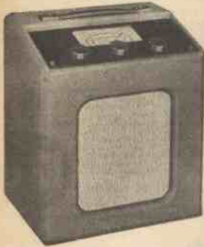
The Vidor self-contained all-battery portable, employing the latest 1.4 volt valves.
