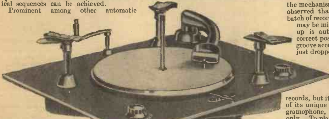
Fig. 8.—The Garrard Automatic Record Changer. The records are carried by the three pillars, a quick angular movement of which causes the bottom record to fall on to the turntable.
