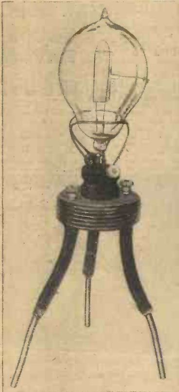
Sir Ambrose Fleming's thermionic valve. This also shows the earliest valveholder improvised in the Swan laboratories.
