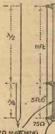
Fig. 5.—The method of end-feeding a half-wave aerial, and (right) a practical arrangement of the aerial.
