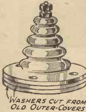
Fig. 1.—The Beehive-type stand-off insulator.
