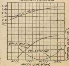
Fig. 2.—This curve shows the relationship between optimum load and harmonic distortion, and also the relationship between optimum load and power output.
