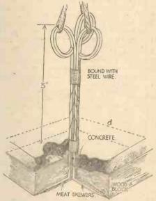
Method of arranging an enchoring look for a vertical single-wire aerial.
