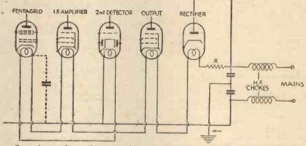
Circuit diagram showing the sequence of heater connections that is generally the most satisfactory for a universal superhet.
