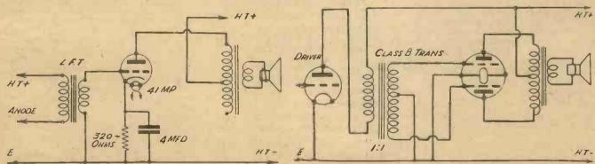
Fig. 2.—A simple L.F. amplifier circuit of conventional type, using a single 41 M.P. valve. Note that the bias resistor has twice the value of that used in Fig. 1.
