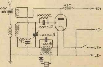
Fig. 3.—The similarity between this simple transmitting circuit and the receiving circuit shown in Fig. 1 is obvious. Aerial and earth are shown broken because these will be replaced by a "dummy". aerial when a full transmitting licence is not held.
