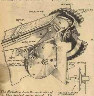
the Ekco flywheel tuning control. The drive has machine-cut gears (40 to 1), and the rim, which is 14in. possible, therefore, that during circumference, permits very accurate settings to be obtained.
