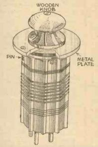
Fig. 2.—A simple plug-in device to ensure easy registration of pins and sockets.
