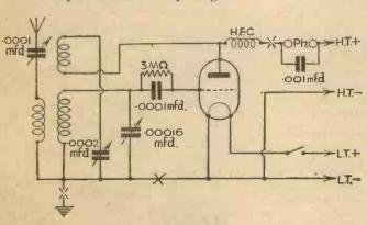
Fig. 1.—A normal type of single-valve S.W. receiver. Points at which audio frequencies can be injected are marked X.
