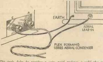
This simple dodge for providing a series aerial condenser is useful when no spare condenser is at hand.
