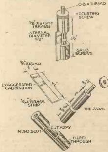
A simple wire gauge, and details of construction.
