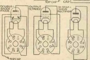
Fig. 2.—Under-base connections for a few typical "International"
