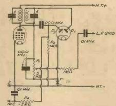
Fig. 5.—Double-diode used for second detection and A.V.C., one anode being employed for each purpose. If desired, a delay voltage can be applied at the point marked X.
