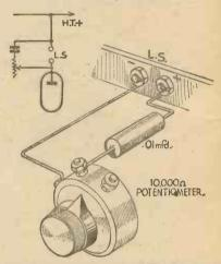
Fig. 2.- A tone control will generally be found advisable with a pentode output valve, a .01-mfd. fixed condenser and a 10,000-ohm volume control being used for the purpose. They are joined across the L.S. terminals, as shown here,
