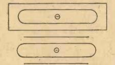
Fig. 1.—Sectional view of two triodes. Although mechanically different they are electrically similar.
