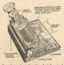
General view of an adjustable coil-winding stand.
