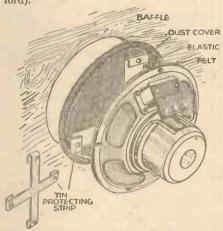
A novel fitment for protecting the cone and spider of a loudspeaker.
