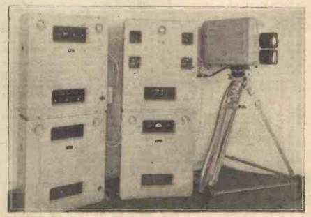
A typical example of continental television practice showing the electron camera and associated racks used for operating purposes.
