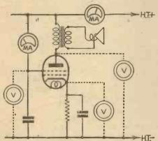
Fig. 1.—Testing a mains output pentode.
