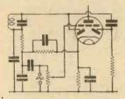
Fig. 70.—The simplest method of connecting a pick-up in a double-diodetriode stage.
