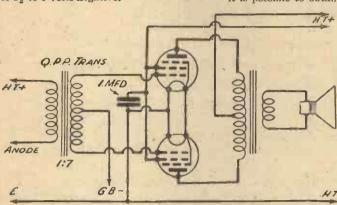
Fig. 4.—This diagrammatic circuit is for two pentodes in Q.P.P.
