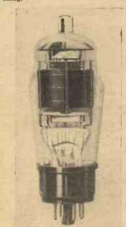
The Hivac All-stage valve, which simplifies receiver design, as it may be used in any stage of a receiver.
