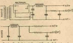
Fig. 1.—Standard circuits for an A.C. and a D.C. mains unit.
