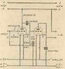
Fig. 3.—A two-triode amplifier in which both stages are resistance-capacity coupled.
