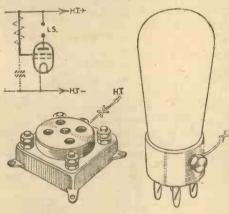
Fig. 1.—An output triode may be replaced by a pentode or tetrode as shown here. In some cases it may be preferable to include a resistance in the additional H.T. lead as shown in broken lines and by the "X" in the above sketch, joining a 2-mfd. condenser to earth, as shown.
