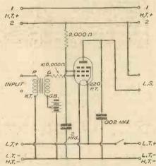
Fig. 2.—How a resistance-fed transformer can be used in a circuit similar to that in Fig. 1.
