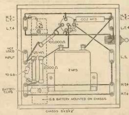
Fig. 4.—Practical wiring plan for the circuit in Fig. 1.
