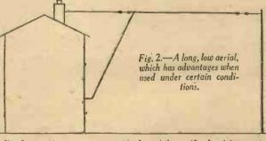
use a vertical aerial, or the lead-in section of the arrangement shown in Fig. 2. Such an aerial will be non-directional, and when the house is situated near or by the side of a main road it will be found that interference from car electrical equipment will be reduced to a minimum, and if any electrical signs are nearby they also will be reduced in intensity if not removed entirely by the use of a vertical aerial.
