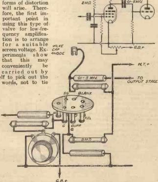
Fig. 2.—The same circuit as used when a battery valve is employed.
