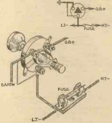
Fig. 4.-When a variable-mu valve is used, as rig. 4.—When a bardote-ma babe is used, as shown in Fig. 3, the existing two-point on/off switch may be replaced by a three-point component adopting the connections shown above. In some cases the H.T.— lead may be joined direct to earth. The original two-point connections are indicated by the broken line.
