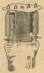
Fig. 2.—A typical triode; note the close spacing of the electrodes. The filament is held at each side by insulated hooks to keep it taut.
