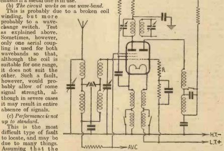
Assuming that the Assuming that the L.F. and detector Fig. 6.—Circuit diagram incorporating a battery triode-pentode frequency changer (Mazda T.P.22).
