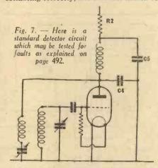
carried out at various points of the dial, a large change in anode current occurs if the grid is touched by the hand. If the valve does not oscillate, it means that the reaction winding is not correct. First try increasing the oscillator anode volts, and then reversing the oscillator anode and grid
