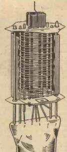
indirectly 4. -Anheated pentode, the Cossor 402 Pen; the relatively close spacing of all three grids can be clearly seen. Observe the open nature of Observe the open nature of the suppressor grid and also swings the anode the box cooling fin at the to a low volend of the grid supports to tage.
