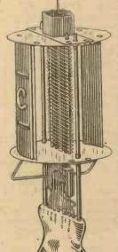
Fig. 3.—A well-designed output tetrode, the Cossor 42 OTDD; note the close spacing of cathode, control grid and screening grid, and the remote, position of the anode.
