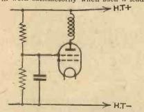
Fig. 4.—How to obtain the screen voltage by means of a potentiometer.
