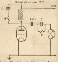
Fig. 4.—Circuit for obtaining a peaked response when using phones.
