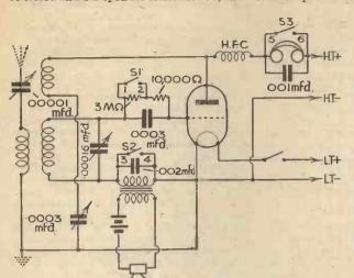
Fig. 4.—How receiver and transmitter circuits can be combined by using frequently used on the 5-metre band (to use which for trans-
