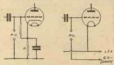
Figs. 71 and 72.—Connecting a pick-up in a detector stage - using a mains and a battery valve.
