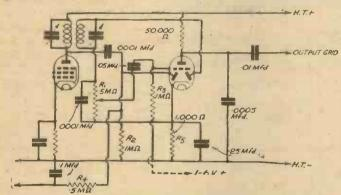
Fig. 6.—Here a double-diode-triode is used for second detection, A.V.C., and first L.F. amplifier. The general arrangement is similar to that in the preceding circuit.
