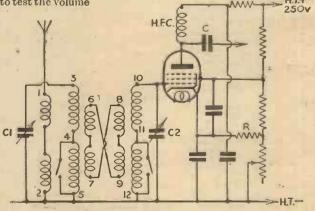
Fig. 3.—A typical H.F. stage with band-pass tuning employing a pariable-mu H.F. pentode (mains type).
