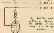
The units of this type should work quite satisfactorily if the receiver is provided with a single lead feeding only the screen or the detector. In some circuits, however, it may be found that the screen of the H.F. valve is joined to the lead feeding the anode of the detector valve, and although the set will work satisfactorily when such a lead
