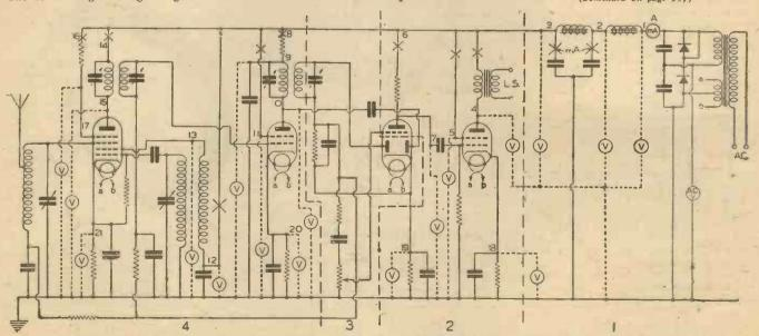
Fig. 17.—Circuit of a simple A.C. Mains superhet indicating the points at which voltage and current tests should be made.
