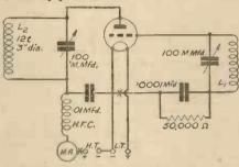
Fig. 6.—Circuit of the inexpensive transmitter described in a letter from Mr. V. H. Thomas.
