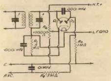
Fig. 4.—A usual form of double-diode circuit for detection and delayed A.V.C.
