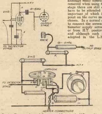
Fig. 1.—The circuit for an A.C. mains amplifier using the H.F. pentode as an L.F. amplifier.
