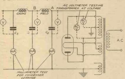
Fig. 16.—Testing a valve rectifier and its smoothing circuit.
