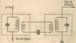
Fig. 1.—Circuit showing the principle of an I.F. filter In the same way the condenser coupling the first detector to the I.F. stage of a superhet. across the primary of the output
