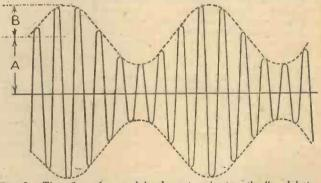
quency corresponding Fig. 2.—The effect of a modulated carrier showing the "modulation envelope.
