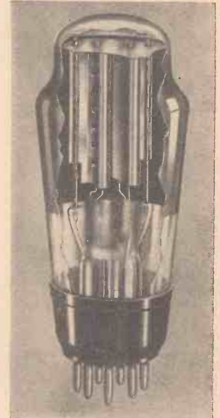
Fig. 3.—A typical Cossor voltage-doubler valve.
