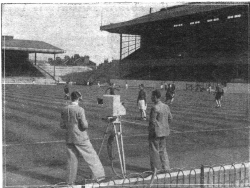
An experiment unique in the history of television and of football was made at the Arsenal ground recently when one half of the team watched by television the other members undertaking their routine training. From the mobile television unit in the Stadium, the pictures were transmitted to the Alexandra Palace, and from there were re-radiated on the normal television wavelength and picked up on a Marconiophone television receiver in the Directors' room in the East Stand.
