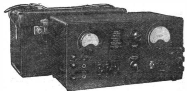
The new 'G.E.C. portable "level" meter.
