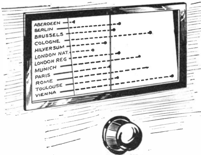
Fig. 2.—Another interesting suggestion for a dial in which a list of stations is arranged alphabetically.
