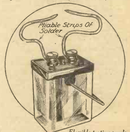
Flexible testing prods for use in connection with a flashlamp bulb.
