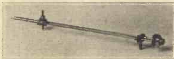
Fig. 1.—A well-made trammel with screw adjustment for marking out scanning discs.
