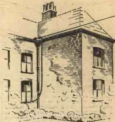
Fig. 1.—Aerial and lead-in running close to gutter and rainpipe.
