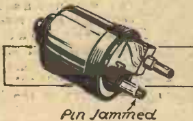
Fig. 3.—A jammed contact pin causes bad contact.
