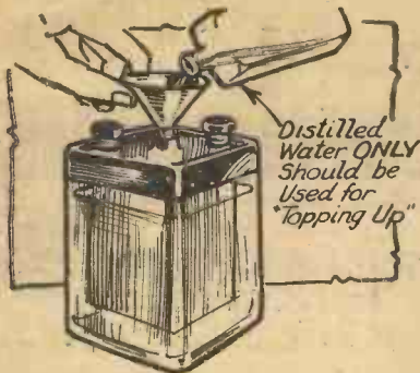
Fig. 4.—Never add acid when "topping" up accumulators.
