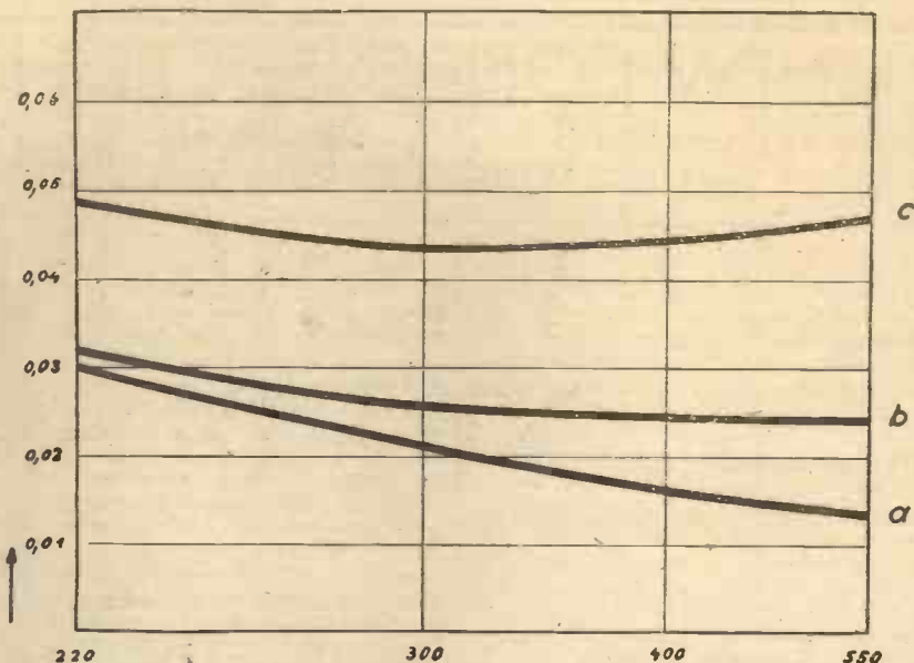
Fig. 8.—Damping curve of: (a) an air condenser. (b) a Vogt flat condenser. (c) a hard paper condenser.
