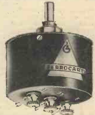
Fig. 6.—A highly selective rejector circuit embodying a Ferrocart coil and a Vogt flat condenser.
