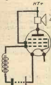
Fig. 2.—A direct anode connection.
