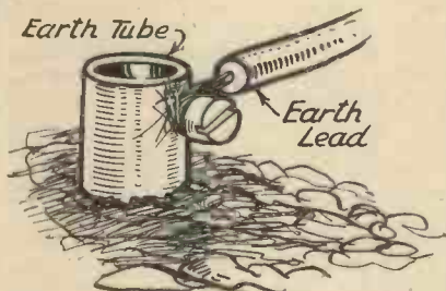
Fig. 7.—Make sure the earth connection is sound.
