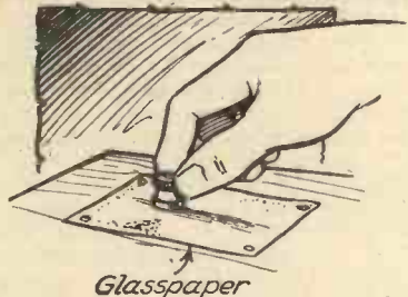
Fig. 1.—Getting a flat and clean surface on a terminal.
