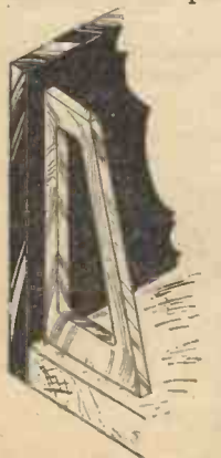
A neat panel bracket made of plywood.
