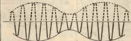
Fig. 3.—The result of half-wave rectification—the "negative" half-cycles have been suppressed.
