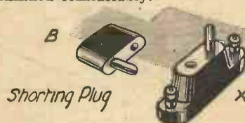
Fig. 3.—The shorting plug.
