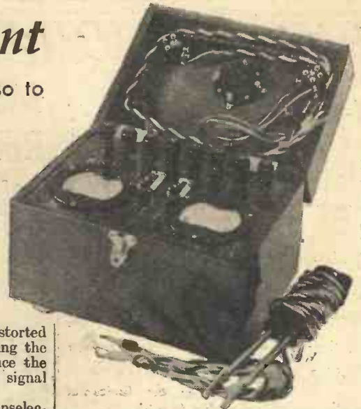
Fig. 1.—A good multi-purpose test set for carrying out measurements on a set to ensure absence of distortion.
