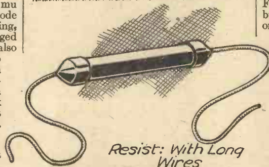
Fig. 3.—Longer wire ends to resistances.
