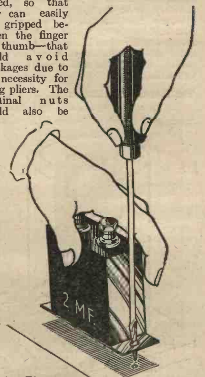
Fig. 3.—The condenser should be lifted with one hand to support the screw.
