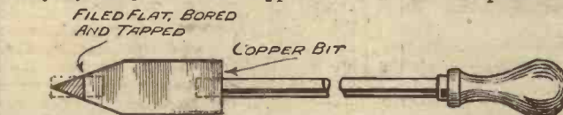
A Muntz Metal tip, added to a soldering iron, facilitates soldering.
