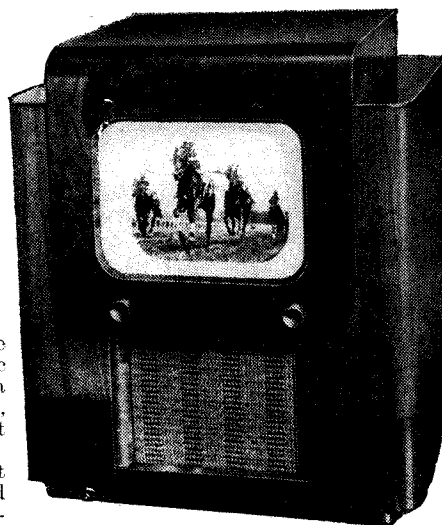
A typical television add-on unit, providing only the television sound and picture.
