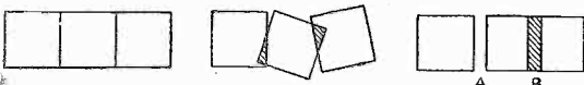
Figs. 2 and 3.—These sketches illustrate the light patches which will be obtained by any overlap caused by inaccurate aligning of adjacent holes.
