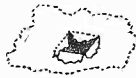
Fig. 4.—The irregular hole which is obtained if the hole is punched against a yielding substance.
