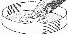
Fig. 3.—After the fluid, the tip is pressed into some solder, until the point is bright all round.
