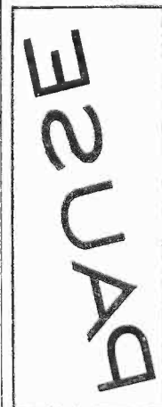
Fig. 1.—Indicating how a word transmitted by television from Germany would appear on a standard English Television receiver.
