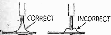
Fig. 7.—The solder should pile up as shown on the left. If it appears as shown on the right the joint is dry-soldered and therefore unsound.
