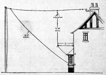
Fig. 3.—A dual aerial, A=S.W. aerial: tead-in at top right-hand side of window. B=B.C. aerial: lead-in at bottom left-hand side of window. C=2 ft. minimum.
