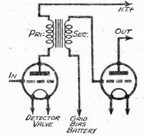
Fig. 10.—The commonest connecting an intervalve transformer.
