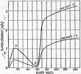
Fig. 2.—Plate volts-plate current curves for an S.G. valve. 500 M C2 ACROSS +10-70v +50v CI I MFD. H.T.+ HT-, LT-, GB+ G.B.-6v. SWITCH
