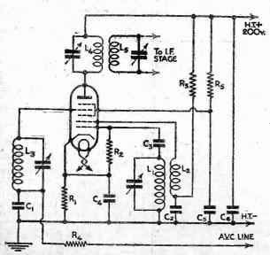
Fig. 3.—The circuit of the pentagrid frequency changer. Rs is not mentioned in the text as it is merely to drop the 200v. to a lower value for the screen grids.
