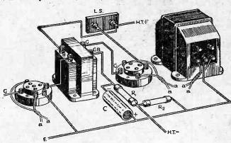
Fig. 8.—A good method of biassing a directly-heated valve which is used along with other indirectly-heated valves and whose cathode (or filament) is heated from the same source.
