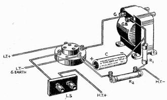
Fig. 3.—G.B. and decoupling resistances in a batteryoperated output stage. R.1 is for decoupling and works in conjunction with the electrolytic condenser C.
