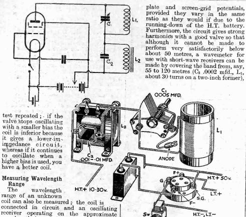
Fig. 4.—By using the circuit shown above, where an iron-core choke is connected in series with a tuned H.F. circuit, the oscillator will oscillate at both high and low frequencies.
