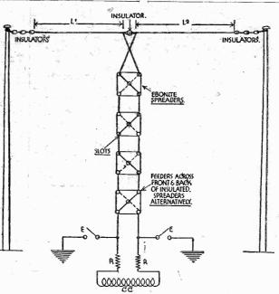
Fig. 5.—Transposed or horizontal doublet aerial. E= earthing switches. CC=coupling coil. RR=600 ohr resistances.  $L^1$ ,  $L^2=40$  ft. aerials.
