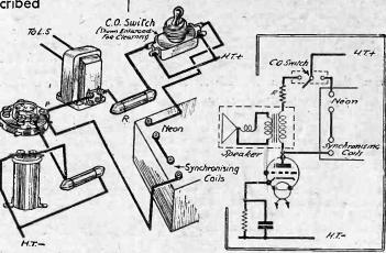
Fig. 1.—The method of switching from "sound" to "vision" when the opparatus is wired in series with the anode of the output valve.
