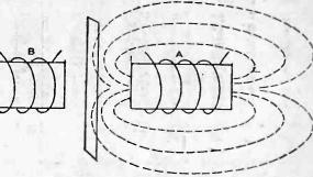
Fig. 3.—Employing an iron screen to " protect " B.
