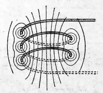
Fig. 5.—The magnetic field round a coil of wire.
