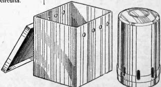
Fig. 4.—The screening box and " can."
