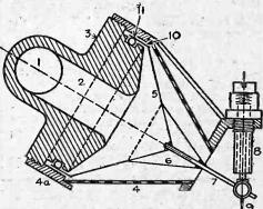
Fig. 2.—1 is an acoustic duct, leading to 2, Pig. 2.—1 is an acoustic duct, leading to 2, Duct in tone arm forming first part of acoustic tube. 3, Main Casting. 4, Conical guard (perforated metal) held by 4a, Screwed ring. 5, Conical diaphragm or "piston." 6, Conical piston extension. 7, Piston rod, connecting to 8, Needle holder, and 9, Needle. 10, Piston skirt, supported by 11, India-rubber rolling ring or obturator. ring or obturator.
