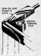
Method of removing broken terminals accumulators
