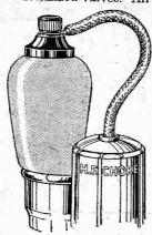
Fig. 6 .--Using a screened wire for connection to the anode cap of an S.G.
