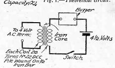
Fig. 5.—Method of using a buzzer to provide oscillations.
