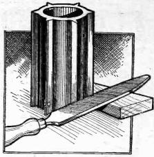
A method of slotting ribbed coil formers.
