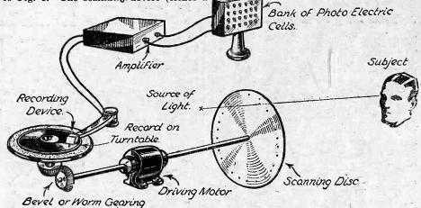
Fig. 1.—Pictorially illustrating how a record of a television transmission can be made in the studio.
