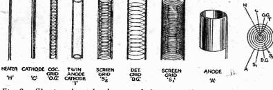
Fig. 2.—Showing the eight elements of the pentagrid valve. There are five grids in all. Note particularly the open structures of the grid marked "T"
