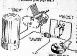
A simple band-pass filter arrangement.
