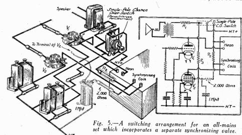
When a Separate Valve is Used for Synchronizing
