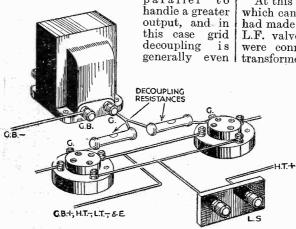
Fig. 2.—Grid decoupling resistances are very desirable when two valves are wired in parallel.
