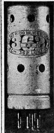
The first all-metal battery valve. This is a product of the 362 Valve Company, and is made under a patented process.
