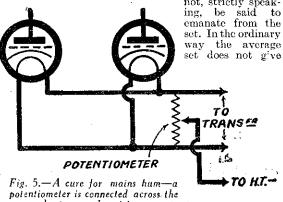
heater supply wiring.
