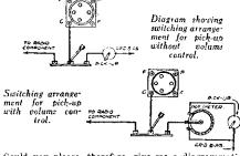
Could you please, therefore, give me a diagrammatic drawing of the switching arrangement for a gramo-phone pick-up? "-(S. V. T., Hastings). The two sketches above show the method of arrang-ing a switch to connect a pick-up to the grid of a valve.
