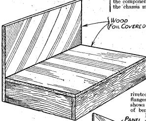
Fig. 1.—A simple way of making a "metal" chassis. A wooden frame-work covered with metal foil.
