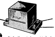
Fig. 2.—How mains hum was introduced into a receiver by a coiled lead in too close proximity to a transformer.
