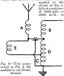
placed across C. This again increases the wavelength of the aerial coil without in-creasing the coupling. In this way the selectivity on the long waves still remains good.
