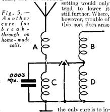
crease the setting of the series aerial condenser and make up for the reduced selectivity by decreasing the coupling between the primary and second-ary circuits. If the coil is a home-made one, this can easily be arranged, either by reducing the number of turns in the tapped portion C, in the case of Fig. 4, or by plac-ing the windings C and D farther apart, in the case of Fig. 5.
