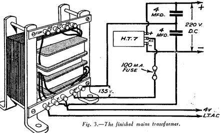
alternatively they may be bought readymade in the form of strong castings from the firms mentioned below. The drawing will need no explanation, whilst the method of fitting the clamps is clearly shown in Fig. 3. This latter drawing also shows the paxolin (or ebonite) terminal strips. These are fitted under the heads of the clamp bolts, and the leads from the spool are brought up to, and soldered to, the terminals.
