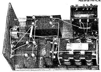
A plan view of the A.C. eliminator, showing the Fig. 4 layout of the components and the wiring.
