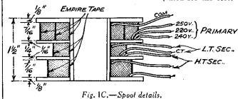
A wooden former having the same cross section as the core  $(1 \ 1/16in. by \ 15/16 \ in.)$ is required and a 1<sup>1</sup>/<sub>2</sub>in. wide strip of cart-Tridge paper is tightly wound round it. Thick shellac varnish is applied liberally to the paper as it is being put on, to stick it and to stiffen the tube. When the tube has been built up to a thickness of about 1/16in. it should be removed from the former and thoroughly dried-preferably by baking in a warm oven
