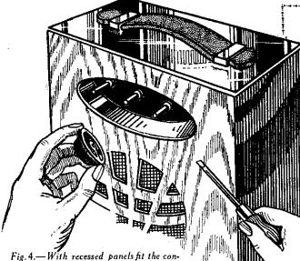
trol knobs before fixing the set into place.
