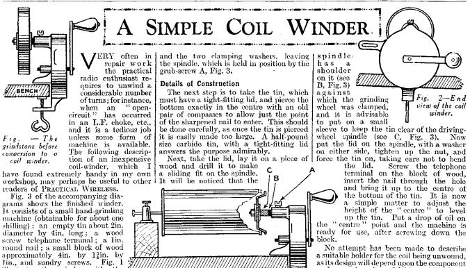
under repair. A useful hint which facili-tates the testing for continuity is to solder the start of the winding to the rim of the tin, then a touch of the test leads on the tin is much easier than looking for the starting end each time.
