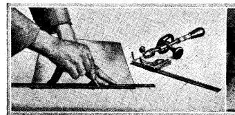
Fig. 7.-Marking the metal with steel straight edge and scriber.
