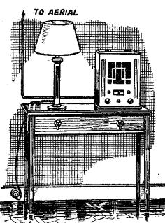
Fig. 8--One cause of hum is the aerial, earth or speaker leads, running parallel to the supply mains.
