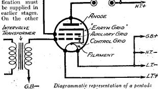
output valve, showing connections.
