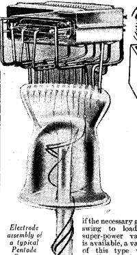
Output Valve. if the necessary grid swing to load a super-power valve is available, a valve of this type will handle it, and give full volume and ex-
