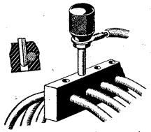
Simple method of tapping short-wave coils.
