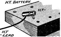
Fig. 3.-The Belling-Lee type of fuse. tension supply. Actually it could be fitted in either the positive or negative high-tension lead, but it is generally inserted between H.T. and L.T. The simplest way to fit a fuse to a set not so equipped is to employ one of those combined with a battery wander plug. It is then only necessary to replace the negative H.T. wander plug by the combined plug and fuse. This type of fuse has the further advantage of being readily accessible. (See Fig. 3.)
