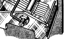
Fig. 9.--Don't let connecting wires foul the condenser vanes.
