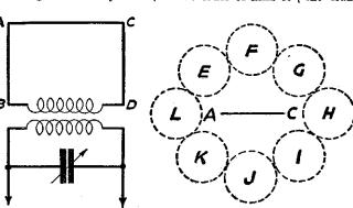
Fig. 3.-The frame acrial with its small coil coupled to the main tuning circuit.
