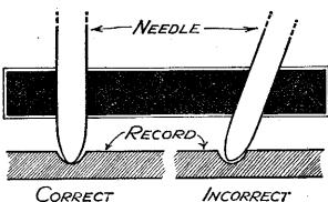
This illustration shows the effect of a needle which is not vertical.
