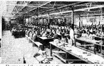
Showing part of the main shop in the new modern factory of Belling and Lez, Ltd. In the foreground can be seen clamping and eyeletting presses, and on the left a power bench. In the background, just right of the centre, is a large battery of capstans. The whole resources of this factory are devoted to the manufacture of Belling-Lee specialities, 90 per cent. of which are absorbed by the radio industry.
