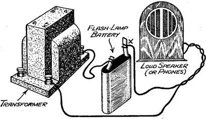
Fig. 2.—The way to test a transformer winding.
