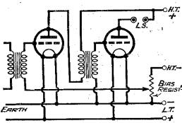
Fig. 6.—A common resistance connected up to provide bias for two battery-heated valves.
