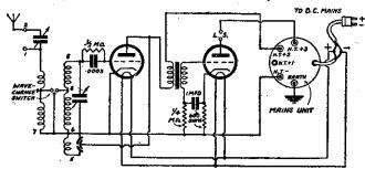
Fig. 2.—The circuit shown by Fig. 1 modified to suit the new Universal full mains voltage valves.
