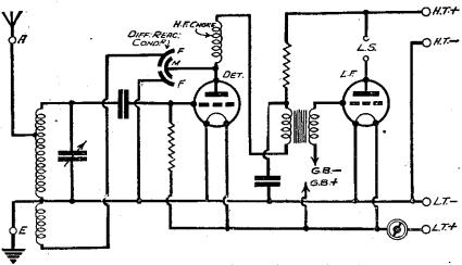
Fig. 2.—Circuit of a two-valve receiver.
