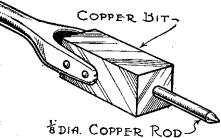
How to fit a small bit to your soldering fron.
