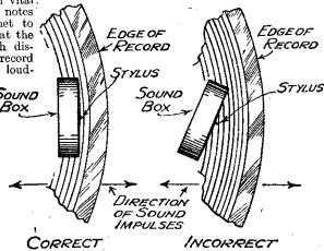
same The "tracking" angle-which was fully explained in a recent strength as the higher notes issue. Note how the sound-box or pick-up must be parallel with the sound grooves.
