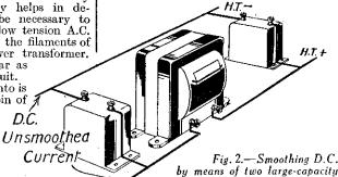
to the choke is a great deal more smooth. The choke in its turn does the work of opposing current fluctuations, passing on a still more steady flow to the second condenser; this is the final reservoir from which the high tension is derived for the set. Usually the inductance value of the choke is not less than 30 henries and the capacity of condensers at least four micro-farads each.
