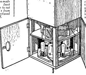
Fig. 6.—Rear view of the completed cabinet, showing set and batteries.
