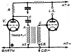
Fig. 2.—The method of parallel-feeding a transformer.
