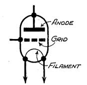
Fig. 3.—Conventional diagram of a threeelectrode valve, indicating the essential parts.
