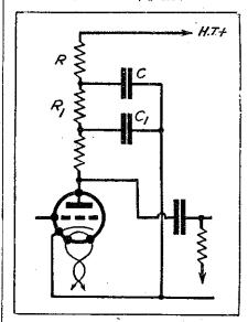
Fig. 6.—R.C.C. stage with double decoupling by resistance R and R1, C and C1.
