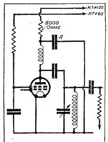
Fig. 4.-S.G. stage decoupled.
