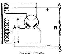
halves of the wave are rectified, although the resulting voltage is only equal to that developed between the centre tap and one end of the winding, or in other words, half the voltage developed across the whole windings. winding
