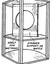
Fig. 2.—The main framework of the corner
