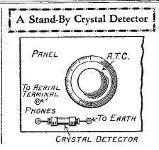
The crystal detector, together with two telephone terminals, can be mounted permanently on the panel, as shown in the sketch, one terminal being connected to the aerial terminal of the set, and the other to one end of the crystal detector. The other side of the crystal detector is connected to the earth terminal.
