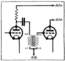
Fig. 2b .- Parallel-fed transformer. With this arrangement no battery current passes through the primary.
