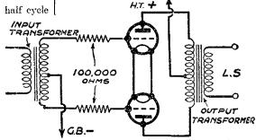
The circuit arrangement of push-pull valves, showing the resistances arranged for ensuring stability.
