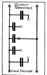
Fig. 1.—How to arrange a number of fixed condensers across the output terminals to vary the tone.
