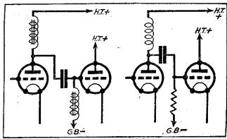
Fig. 3.—Two forms of choke coupling.
