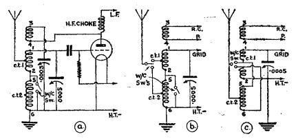
Fig. 2.—Three methods of connecting the tuner shown in Fig. 1 into a detector circuit.
