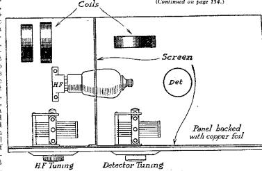
Fig. 2.—A screen the same depth as the baseboard is used for "partitioning of " the H.F. stage.
