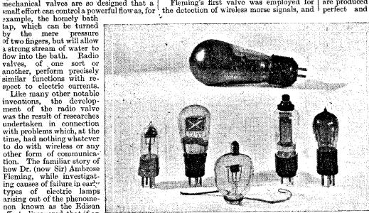
Fig. 2.—A group of Cossor valves indicating various stages in development. Typ. 2.—A group of Cossor valves inalcating various stages in accessment. Top: Super-power valve of 60-Watt dissipation. Bottom row (left to right): (1) 1921—6 power valve, Stentor class. (2)—Modern pentote. (3)—1916 valve of peculiar construction. (4)—Modern mains S.G. valve (5) 1923—.3 amp. kalenised filament.
