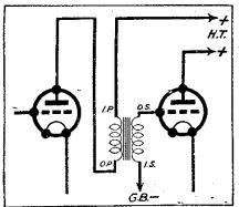
Fig. 2a.—Transformer primary directly in anode circuit.
