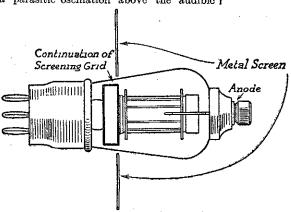
Fig. 3.-The screen should be level with the screening grid of the valve.
