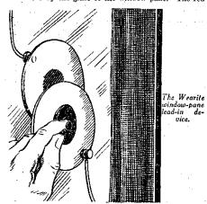
disc is stuck outside the window, and the lead-in attached to the clip on this disc, whilst the other disc is fixed inside the window, and a lead taken from this to the aerial terminal of the receiver. The device thus saves drilling a hole and at the same time serves as a series aerial condenser. The capacity may be
