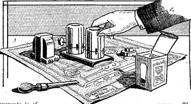
alternatives to those specified in the list. In this case it is usual to mount the components with the terminals in as nearly the same position as those shown on the print. This may mean turning the component round. However, in the case of unshielded coils or chokes it is better to lengthen or shorten the leads rather than alter the position of the components in relation to others.
