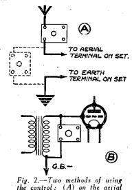
the control: (A) on the aerial circuit, and (B) across a transformer.
