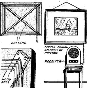
Figs. 5, 6 and 7.—A picture frame can be easily adapted to accommodate an aerial.
