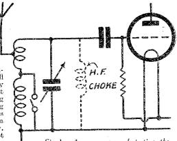
Fig. 1.—An easy way of testing the efficiency of an H.F. choke is to connect it across the tuning coil of your receiver.
