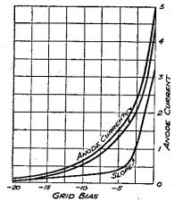
Fig. 1. The characteristic curve of the variable mu value. Note the long, gentle slope caused by the irregularly spaced grid.
