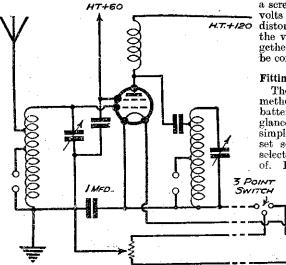
Fig. 2. The method of fitting variable bias to a battery type of variable mu.
