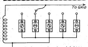
This diagram explains the method of joining up the condensers. The diagram also shows how a number of semi-fixed condensers may be connected up to enable the scheme described in this article to be carried out.
