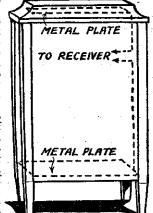
Fig. 8.—A radio-gram cabinet containing aerial and earth plates, direction, then hang the picture on a wall at right angles to the first.
