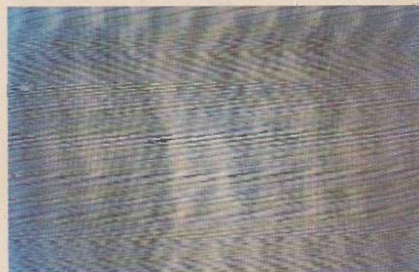
Picture 6: Cross-modulation, caused by excessive signal strength.
