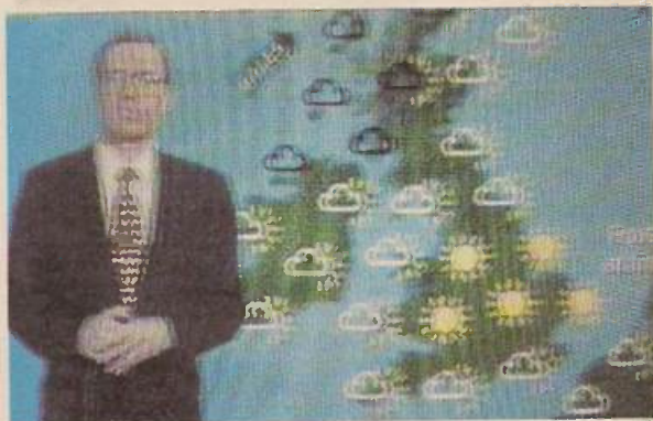
Picture 10: Ghosting, caused by multipath reception.
