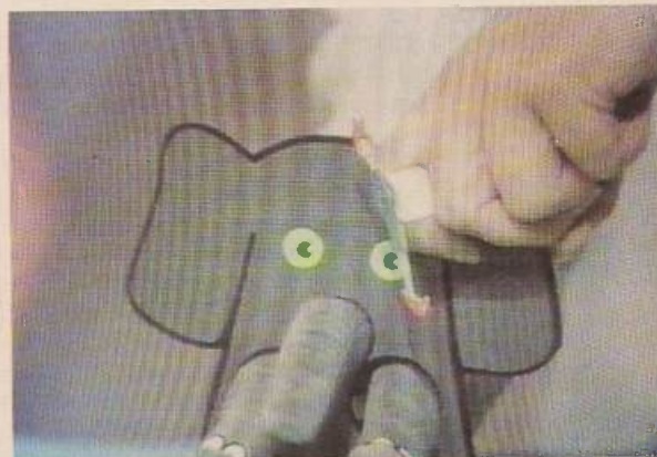
Picture 11: Ringing, another effect produced by multipath reception.
