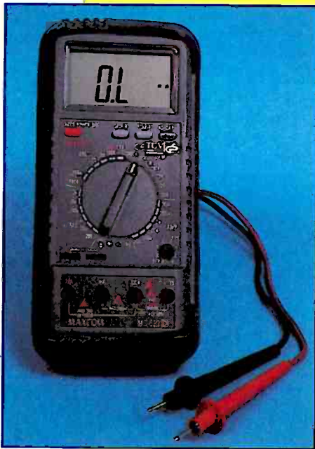
Digital multimeter reads not only voltage, current, and resistance but also capacitance to 200µF, frequency to 20MHz and transistor h_{FE} – all for just £59.
